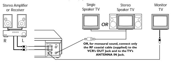
For stereo sound, connect the audio cables to the AUDIO OUT Jacks on the VCR and to the AUDIO IN Jacks on the Stereo Amplifier or Receiver. Then, connect the video cable to the VIDEO OUT Jack of the VCR and to the VIDEO IN Jack of a monitor TV.
